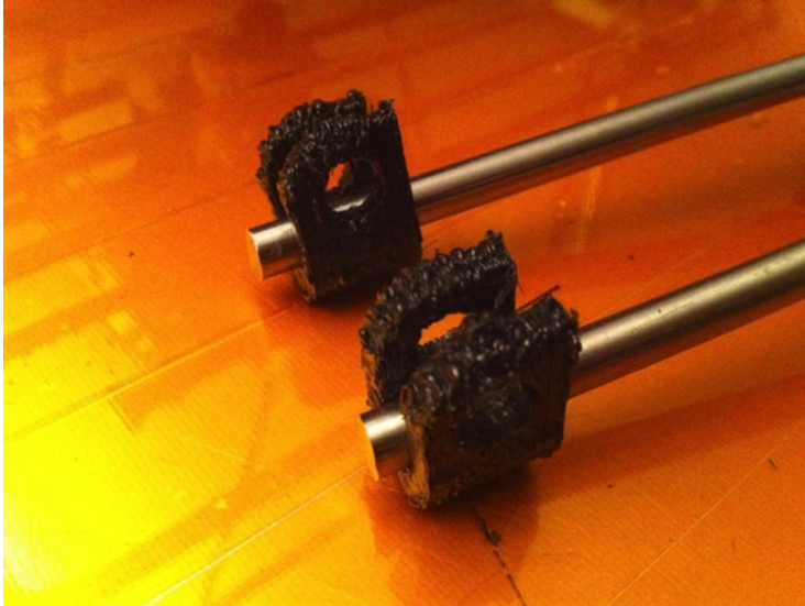
Figure 15-4. The new, stronger clamps I designed. Side note: back then, this was considered acceptable print quality
