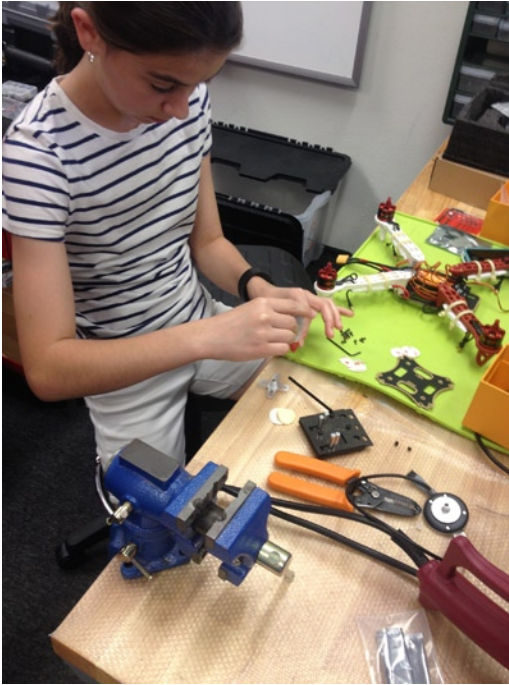
Figure 4-4. A programmable DIY quadcopter being made from parts. Photo courtesy of Mosa Kaleel
