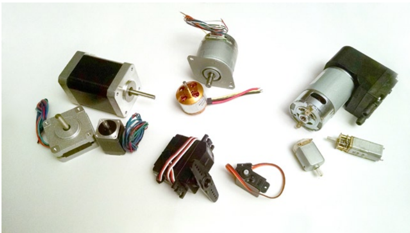
Figure 4-1. Just a few motors from Rich’s collection. Top: brushless. Right: brushed. Bottom: servos. Left: steppers
