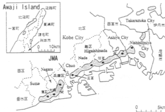
Fig.1 Areas of severe building damage
