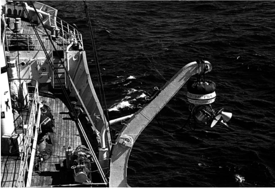
Figure 8.9. Placement of the gyroscope stabilization platform with its highly sensitive radiothermal instruments aboard the RV Mikhail Lomonosov (Black Sea basin, August 1978).
