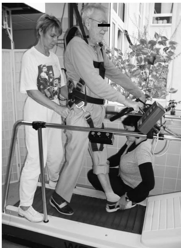
**Figure 18.1** Treadmill training with partial body-weight support. The patient stands on a motor-driven treadmill with variable speed control (range 0.01–2.25 m/s) and is supported by a modified parachute harness suspended by a set of pulleys.
