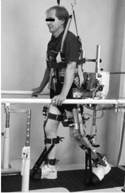
**Figure 18.6** Paraparetic subject practicing on the Lokomat, an exoskeleton with powered drives to bend the hip and knee during the swing phase.
