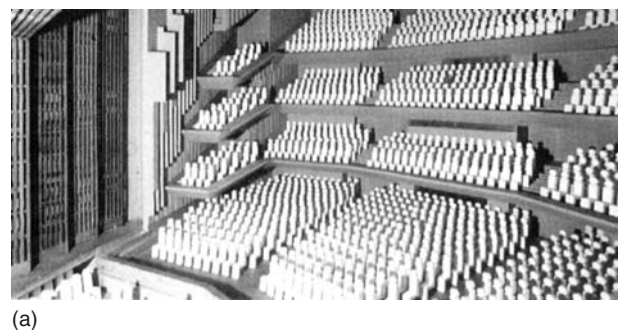
Figure 12.14 Auditorium acoustics. (a) Model simulation. Example of a physical model of an auditorium simulating the acoustic characteristics, by Sandy Brown and Associates.
