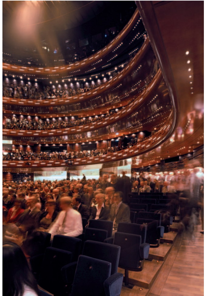
Auditorium. The curved balcony fronts on three levels, with a technical gallery over, containing the house lights and acoustic treatment. Batches of seven LED luminaries occur in the balcony ceilings (a theme seen in the internal and external public spaces).
