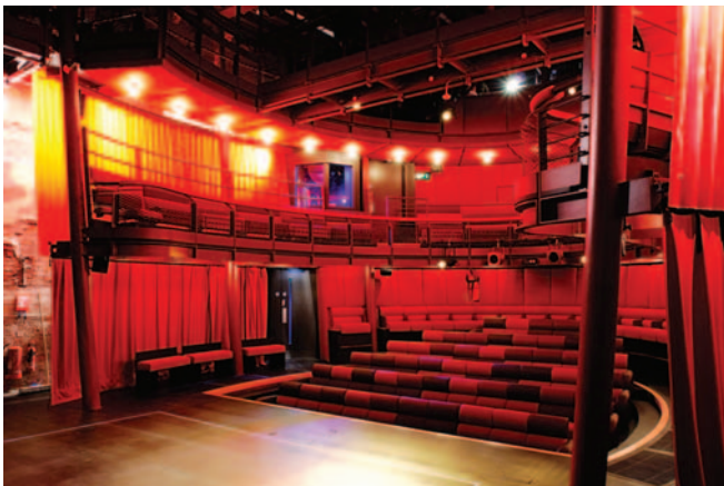
Seating structure detached from inherited stone outer wall Photo: Haworth Tompkins
