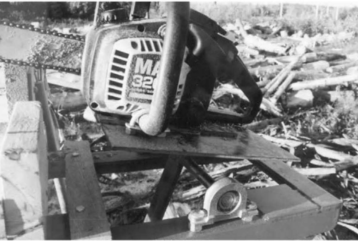
9.4: Pillow blocks make an excellent pivoting mechanism.
