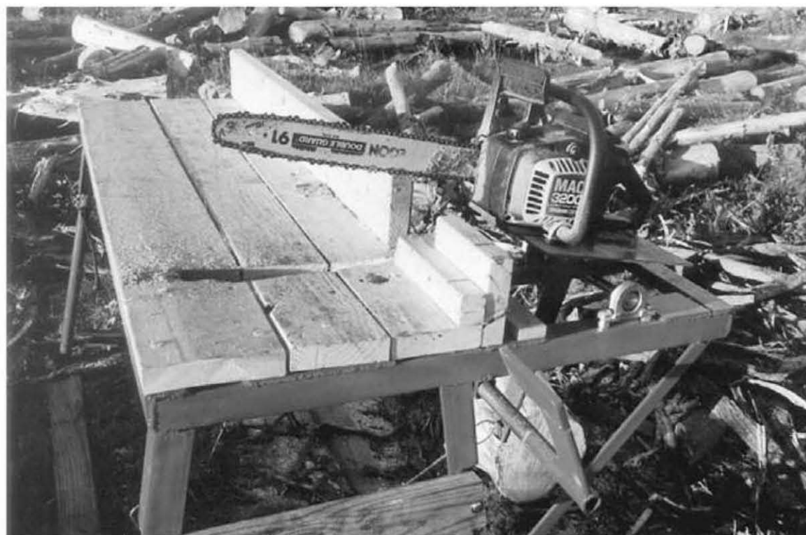
9.6: The Mother's Cordwood cutoff table. Credit: The Mother Earth News. May/June 1982. p. 110.
