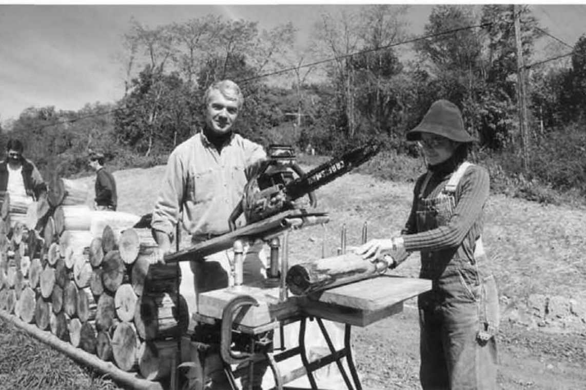
9.5: Charles Shedd of Bakersville, North Carolina used his ingenuity to build this very effective — and portable — cordwood cutoff mechanism.
