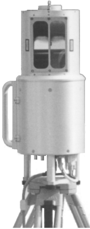
Figure 2.1 Range scanning apparatus used to determine the physical geometry of scenes. The way this device works is quite remarkable (see Besl, 1988). A scanning mirror inside the rotating optical head directs a laser beam over a precise angular pattern. The beam of collimated infrared light is pulsed periodically from the laser, such that each point (pixel) in the scene is evaluated sequentially. The signal reflected back from object surfaces is detected by a photodiode, which in turn produces an electrical “receiver signal”. The tiny interval of time between the transmitted pulse and signal returned is determined by a quartz-stabilized clock; based on the speed of light, the distance from the scanner to each surface point is then calculated by a microcomputer. The distances determined in this way are accurate to within a few millimeters. The spatial resolution (angle step-width) of this process is selectable between 0.072^\circ to 0.36^\circ in both elevation and azimuth. For practical reasons, we chose 0.144^\circ ; at this resolution it takes approximately 3 minutes to scan an image that encompasses the standard “field of view” of the scanner, an acquisition time that works well in the field.
