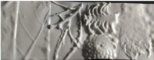
Figure 13.8 thermoformed PLA panel with surface structure. © P. Siedler/ITKE.
