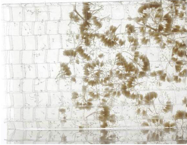
Figure 13.6 Sandwich panel with thermo-pressed cover panels with dried flower inlays. © Damböck/Pixelcatcher.
