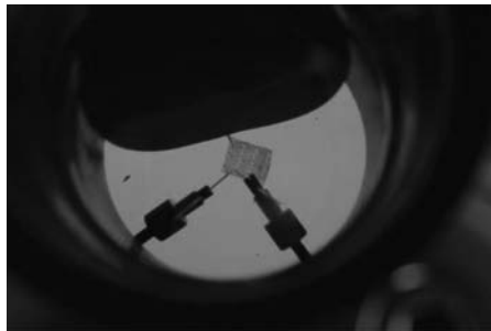
FIGURE 16.9 HEMT device under test at 1000°C in a vacuum chamber.
