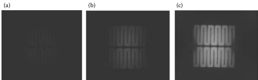
FIGURE 2.12 Microscopic images under applied voltages of (a) 2.28 V, (b) 2.62 V, and (c) 3.00 V, respectively.
