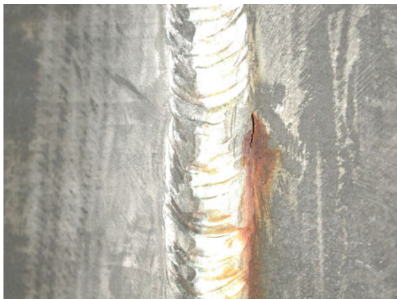
Fig. 4.44 Crevice corrosion under a weld in austenitic stainless steel (published with kind permission of TNO)
