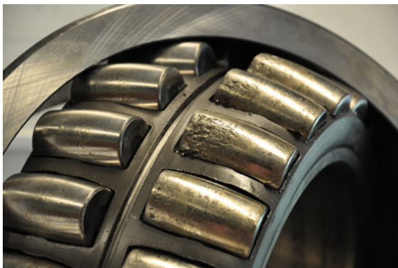
Fig. 4.35 Surface fatigue damage in the rolling elements of a wind turbine bearing
