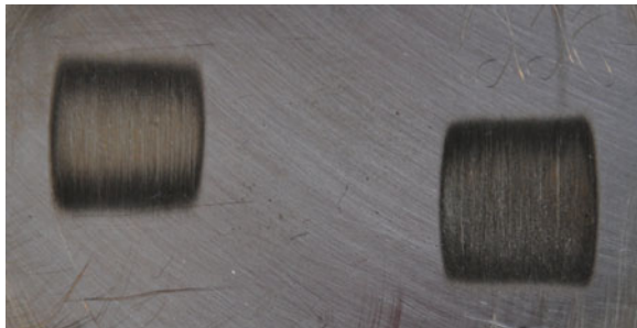
Fig. 4.34 Wear scars due to abrasive wear by sand particles in a rectangular contact
