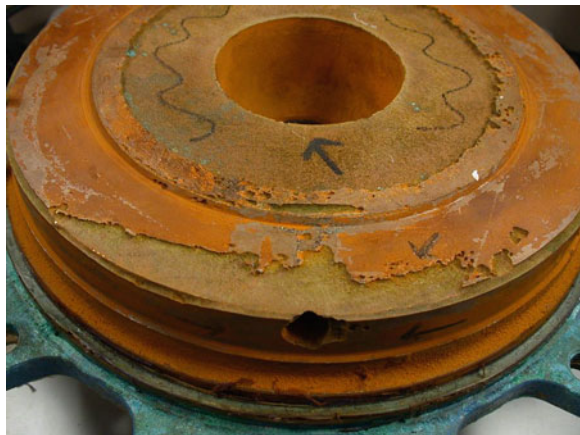
Fig. 4.47 Pump impeller damaged by interaction of erosion and corrosion (published with kind permission of TNO)
