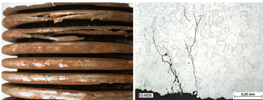
Fig. 4.45 Stress corrosion cracking in austenitic stainless steel component ( left ) and a micrograph showing the development of the cracks ( right ) (published with kind permission of TNO)
