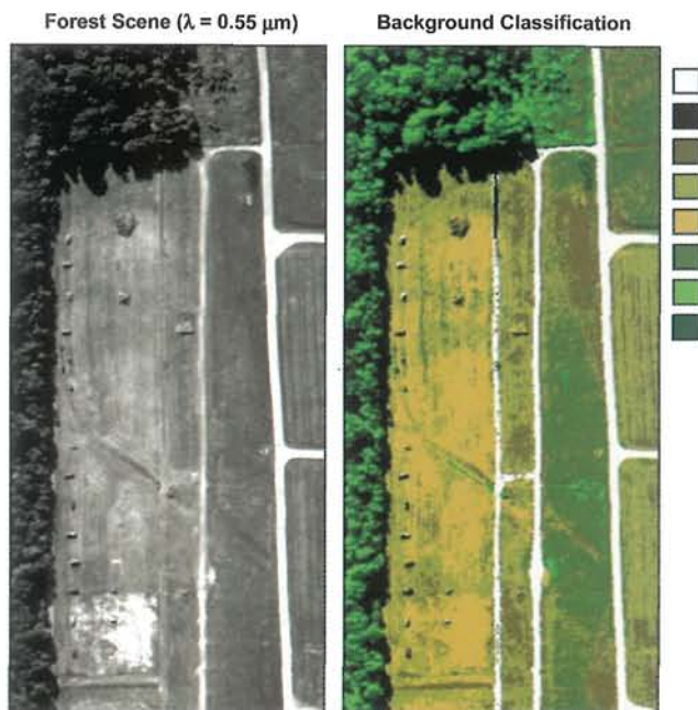
Figure 8. Example background classification. The left panel is a band image at \lambda = 0.55 \mu\text{m} . The right image is the background classification of iso-data clustering based on 5 principal components.
