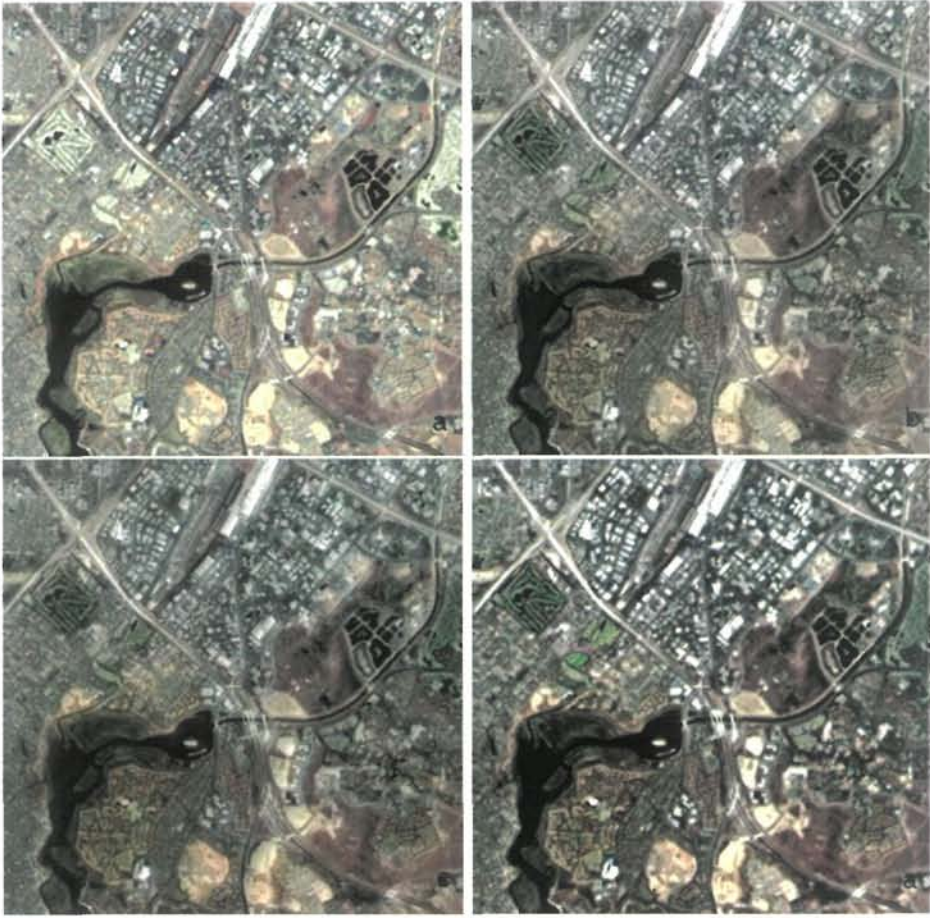
Fig. 9. Merged images from Fig. 3, using a: IHS; b: MERGE1; c: MERGE2; d: proposed technique
