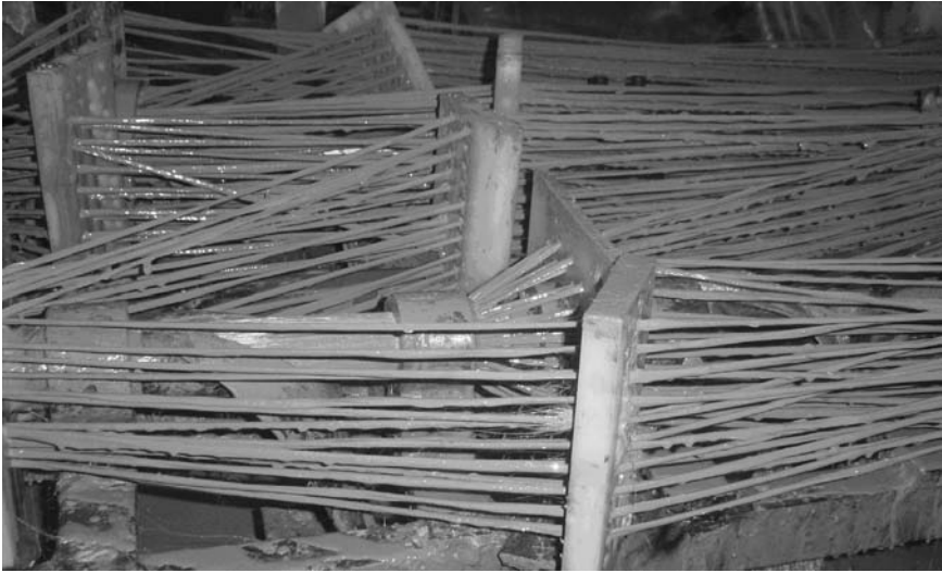
Figure 6.3 Glass fibre drawn through a die and coated with epoxy.
