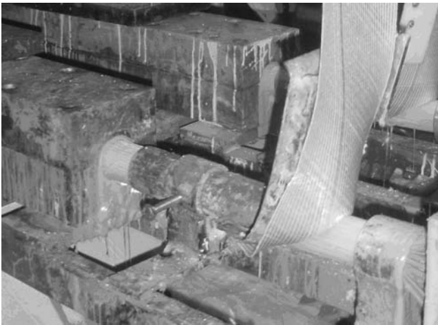
Figure 6.4 Fibre drawn and coated with sheeting to form a pipe bonded with epoxy.
