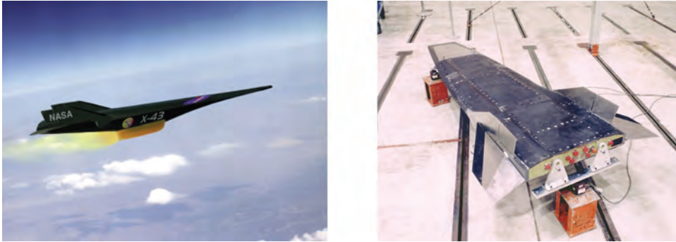
FIGURE 3.8 (Left) Artist's rendering of the X-43 hypersonic flight demonstrator and (right) image of an actual vehicle during assembly. SOURCE: Images downloaded from the NASA Image Exchange Server, http://nixon.nasa.gov/ .
