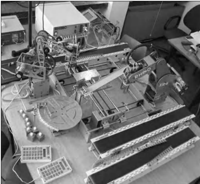
Figure 5.21. The setup of the laboratory MS (a two-robot material-handling cell)
