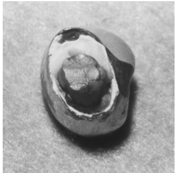
Fig 1-11 Brittle fracture of an amalgam post and core that had supported a PFM crown. Set dental amalgam is a mixture of several intermetallic compounds. Intermetallic compounds tend to be brittle rather than ductile. (Photo courtesy of R. P. O'Connor, DMD.)
