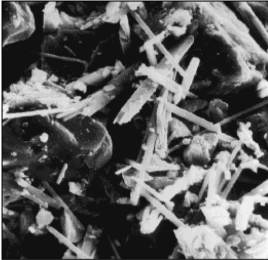
Fig 4-9 Microstructure of a set gypsum-bonded investment (Kerr Cristobalite Inlay; W/P = 0.38). The large particles are cristobalite; the small acicular crystals are gypsum formed during setting. (Scanning electron micrograph of fracture surface, original magnification \times 3,000 .)
