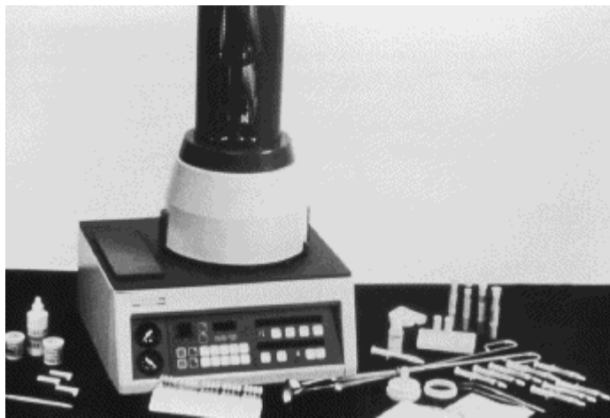
Fig 15-18 Injection-molding oven for high-leucite porcelain.
