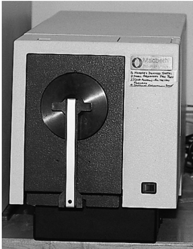
Fig 3-11 Spectrophotometer for laboratory measurement of color parameters (Macbeth 7000, Gretag-Macbeth.)
