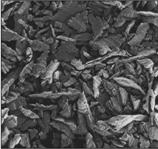
Fig 12-2 Traditional lathe-cut amalgam alloy. (Original magnification \times 100 .)
