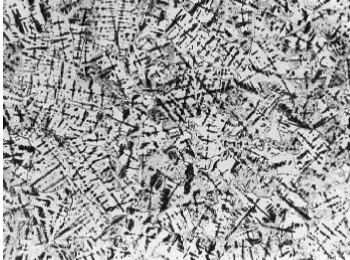
Fig 13-4 Dendritic (skeleton- or needle-shaped) grain structure of precious metal alloy as cast. (Original magnification \times 100 .)
