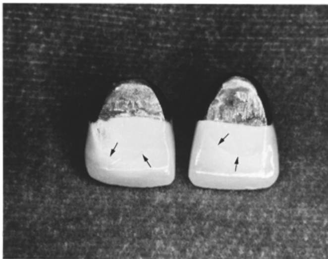
Fig 1-4 Brittle fracture ( arrows ) of ceramic (dental porcelain) due to mismatch in the coefficient of thermal expansion between porcelain and metal. (Photo courtesy of R. P. O'Connor, DMD.)
