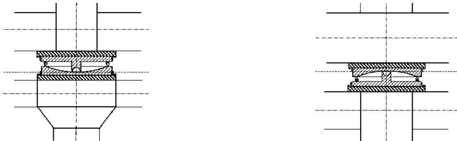
Fig. 6- 15: FPS bearing in downward (left) and upward (right) position.
