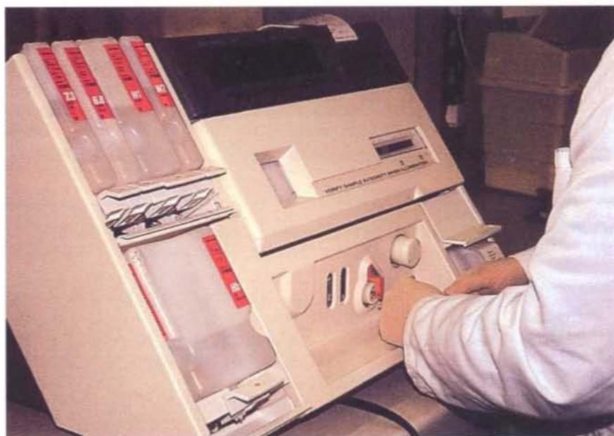
Fig. 1 Blood gas analyzer.
