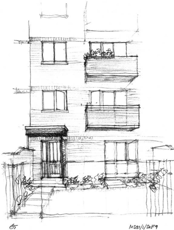
Figure 7.2 Sketch of new maisonette entrances and private gardens in an estate project. The three-dimensional drawing stimulated discussion among users on the correct height of fencing— high enough to provide some privacy, low enough that the surveillance of passers-by could guard against intruders.
