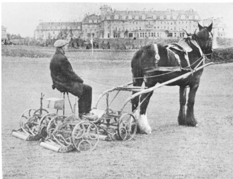
Fig. 2.1 The first Ransomes 'Triple' mower had a cut of seven feet and in 1924 cost £125 (£210 for a quintuple), carriage paid to any railway station. This one is standing in front of the Gleneagles Hotel. The horses normally wore leather boots to reduce surface damage. (Courtesy of Ransomes Sims Jefferies plc.)
