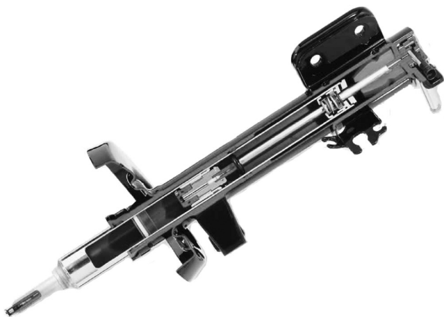
FIGURE 1.8 Photograph of MR shock absorber.
