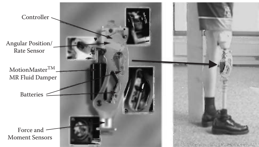
FIGURE 1.9 Photograph of MR damper for a leg.
