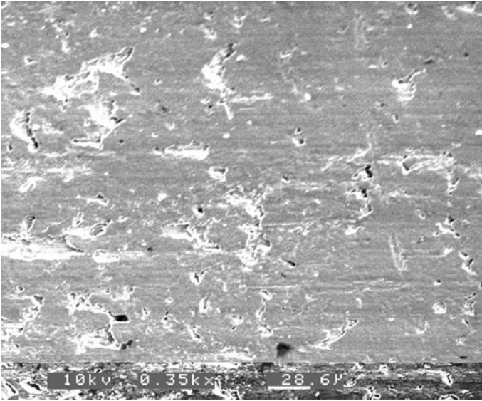
Fig. 2.3 Typical scanning electron micrograph of machined surface, hot-rolled Al/SiC, 20% vol. SiC
