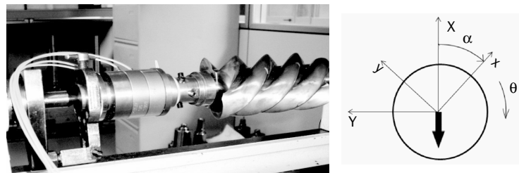
Figure 3.3 Calibration scheme for radial forces and torque
