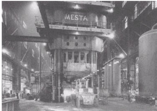
Mesta-built Alcoa 50,000-ton hydraulic forging press, Cleveland, Ohio, in raised position. Photograph by Jet Lowe, Library of Congress Collections.
