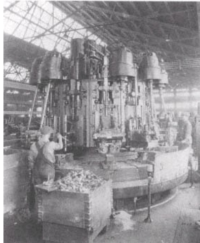
A. O. Smith automatic frame plant. Shown is a special machine for finishing spring hangers.
