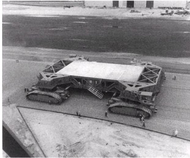
Larger than a baseball infield, the crawler transporter (here, without the thirty-six-story Apollo-Saturn space vehicle it was designed to transport) makes its way along the special roadbed of Launch Complex 39 at the Kennedy Space Center. Courtesy NASA.
