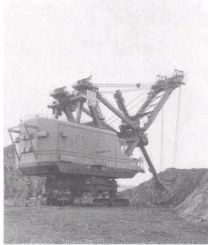
Bucyrus-Erie's "Big Brutus" mine shovel takes a 90-cubic-yard (69 m 3 ) bite of Kansas coal.
