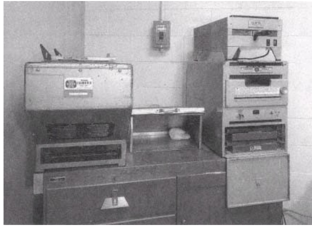
Xerox Model D copier, one of the first production units, at Battelle's Columbus laboratories. Photograph by Jet Lowe, Library of Congress Collections.
