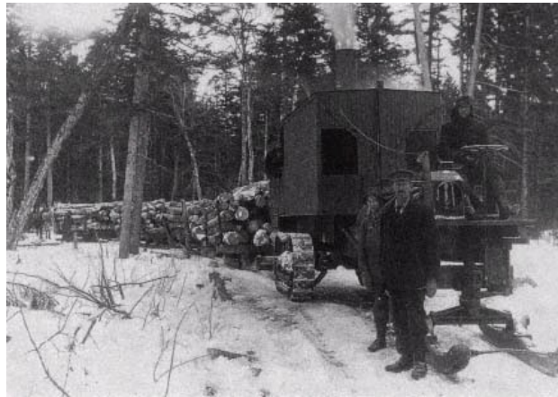
The steam-powered Lombard log hauler, developed by Maine mechanic Alvin O. Lombard in 1900, greatly expanded the area from which timber could be harvested profitably.
