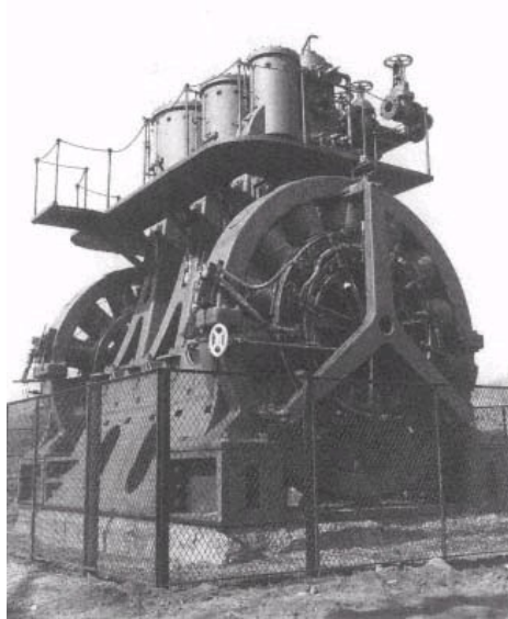
Marine-type, triple expansion, engine-driven dynamo as it appeared in 1989, before its restoration and relocation inside the Henry Ford Museum. Today, the engine and dynamo operate with the assistance of an electric motor.
