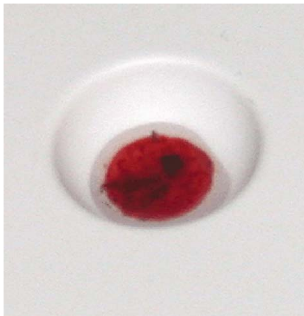
Color Plate 2, Fig. 13. Anatrazoline color test. ( See discussion in Ch. 5 on p. 98. )
