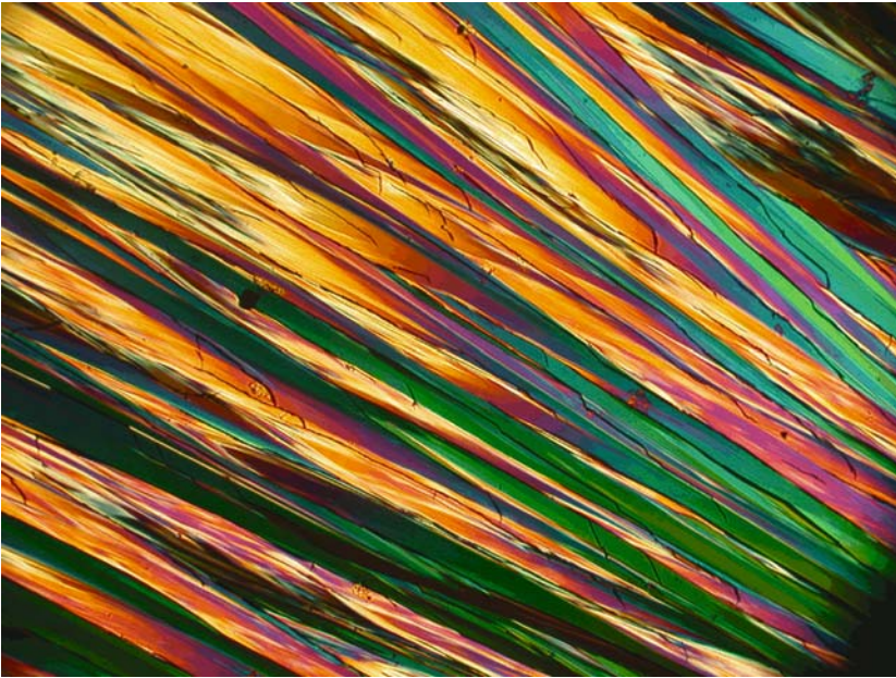
Color Plate 3, Fig. 17. TNT fusion melt. ( See discussion in Ch. 5 on p. 102. )
