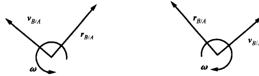
FIGURE 2.4 The direction relationship among the vectors \mathbf{v}_{B/A} , \boldsymbol{\omega} , and \mathbf{r}_{B/A} for planar motion.
