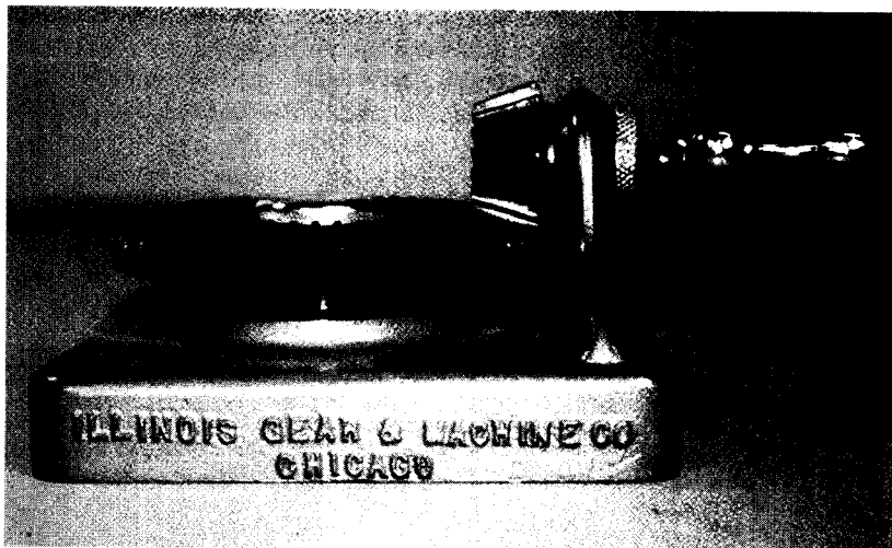
FIGURE 11.17 Bevel gears with 90° shaft angle.
