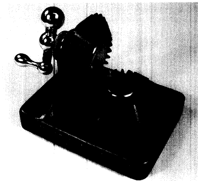
FIGURE 11.26 Miter gear geometry.
