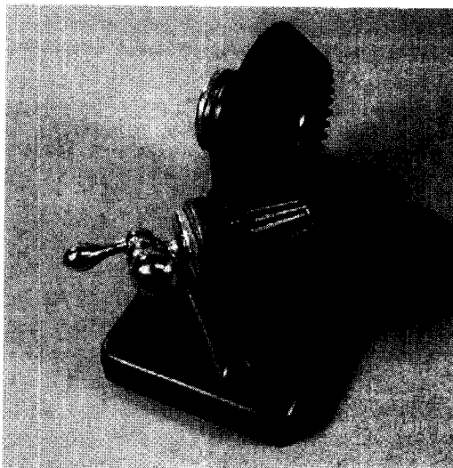
FIGURE 11.29 Angular bevel gear model.
