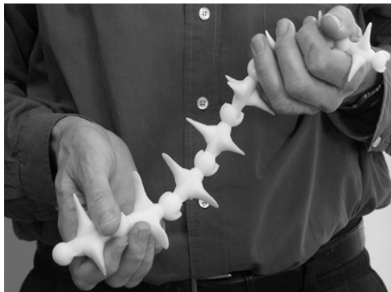
FIGURE 2-8 Object with seven articulating joints from a 3-D printer. Courtesy of the MIT Media Lab.
