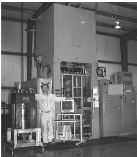
FIGURE 2-7 Computer-driven, powder metallurgy press (foreground) with traditional press behind. Reprinted with permission of Mii Technologies.
