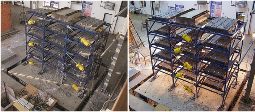
Fig. 3.4 Set-up of MODEL02 and MODEL04 on the shaking table (Rakicevic et al. 2009b)
