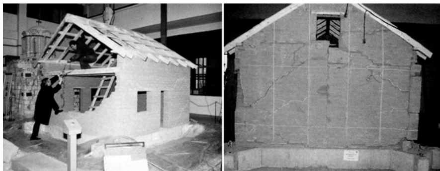
Unretrofitted Adobe Model UAB
