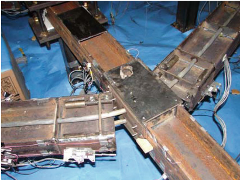
Fig. 19.10 Detailed view of a disintegrated interior beam-column connection of the PTED specimen after the pushdown test
