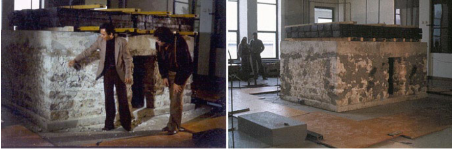
Fig. 12.1 Original and repaired model of a typical building in the old town of Budva
