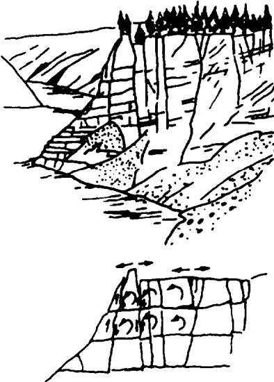
Suggested toppling failure mechanism of the north face of the Vajont slide. After Muller 245 .
