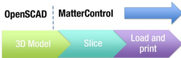
Figure A-1. 3D-printing workflow with OpenSCAD and MatterControl
