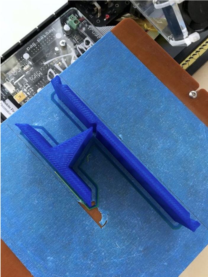
Figure 5-2. Class 1 lever on the printer
