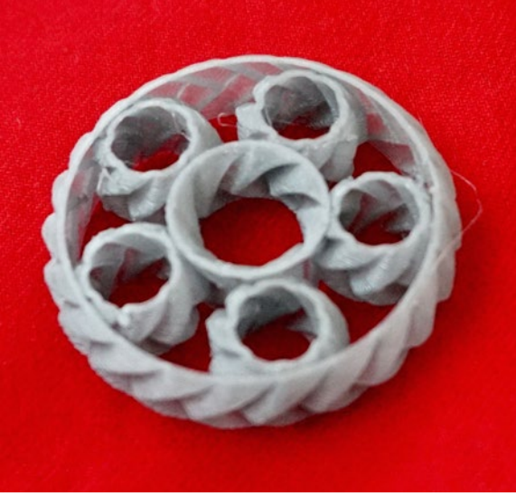
Figure 5-15. Rich's quick print gear (prints assembled, just as shown)
