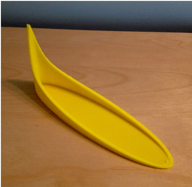
Figure 3-4. Halley’s Comet orbit model. Dots (partially buried in the model wall since the eccentricity is so extreme) are foci, height is instantaneous orbital velocity. The Sun is at the focus at the base of the high-velocity part of the orbit
