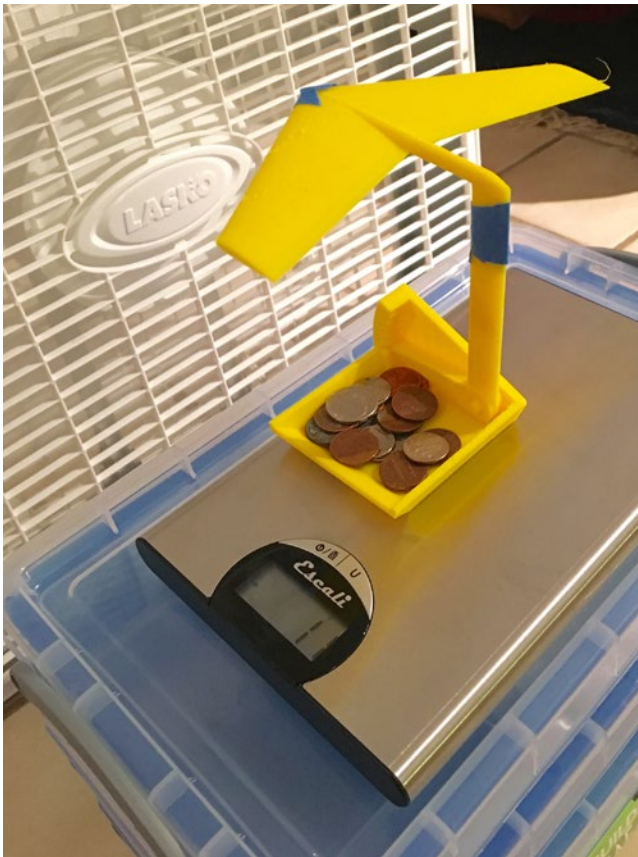
Figure 4-8. Using the output of the model in Listing 4-2 to measure lift
