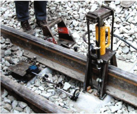
Fig. 6. Test of ballast bed's vertical stiffness
