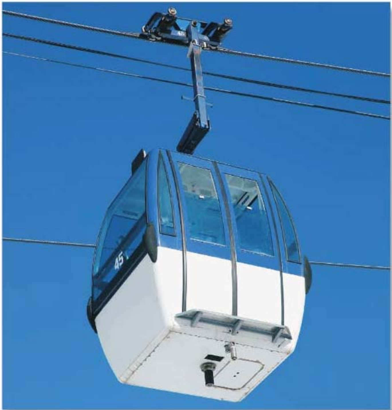
The offset hanger supporting this ski gondola is subjected to the combined loadings of axial force and bending moment.
