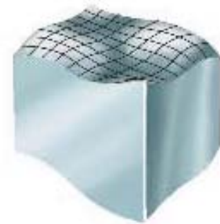
Warping of cross-sectional area
