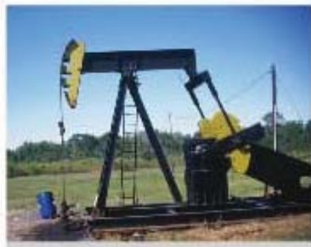
Engineers must account for possible fatigue failure of the moving parts of this oil-pumping rig.
