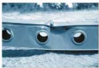
This crane boom failed by buckling caused by an overload. Note the region of localized collapse.
