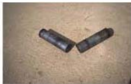
This pin was made from a hardened steel alloy, that is, one having a high carbon content. It failed due to brittle fracture.
