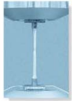
Typical necking pattern which has occurred on this steel specimen just before fracture.
