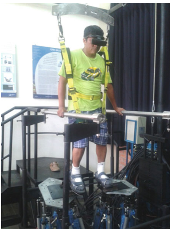
Fig. 7 A lab layout for tests with the prototype of Lima walking simulator
