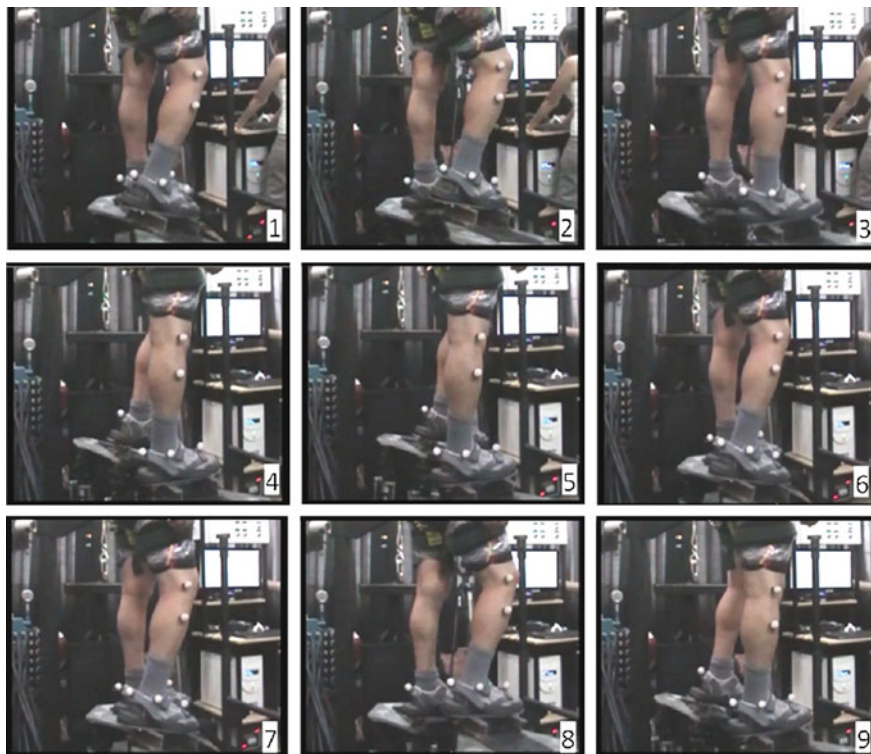
Fig. 8 Snapshot of an on-site walking test with Lima walking simulator
