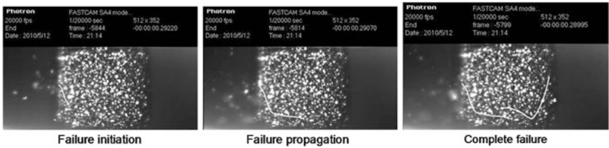
Fig. 6 Typical failure initiation and propagation in end-potted carbon foam specimen
