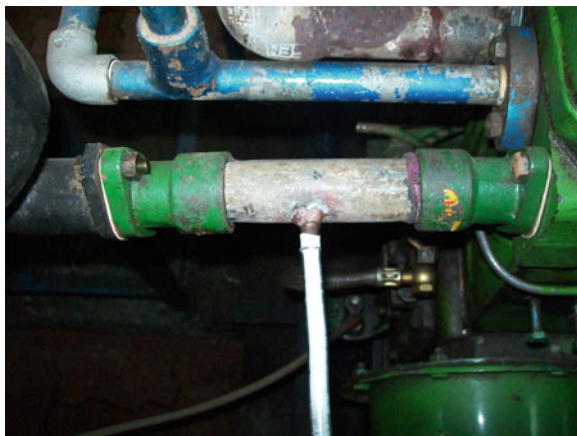
Fig. 2 Modification made to the engine for hydrogen inlet
