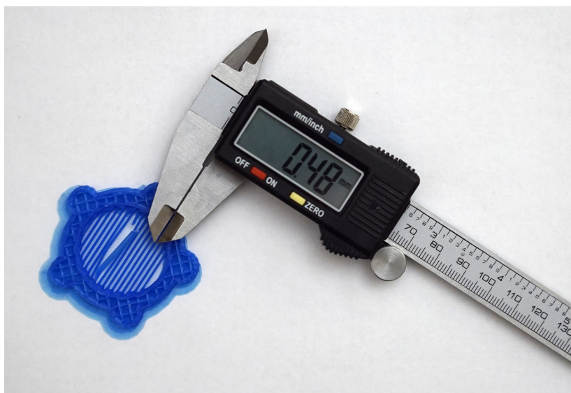
Figure 4-17. Calipers show an extrusion width of .48mm extruded from a .4mm nozzle
