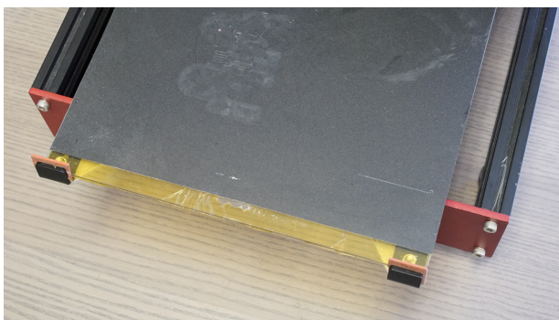
Figure 4-25. Specialized Buildtak adhesive surface applied to the build plate
