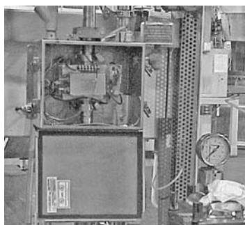
FIGURE 8.31 The sensor of Figure 8.21 is shown here in a milling loop at a pigment plant. The spool piece is mounted directly in a vertical pipe and is enclosed in a nitrogen-purged box (which is open in this photo). The chart shows the signal strength as a function of time for three production lots.
