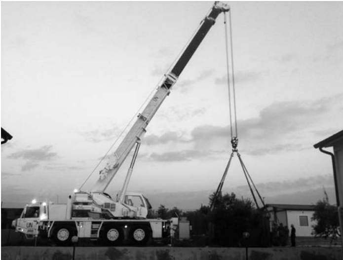
Figure 4-5. An Italian Mercedes 30 metric tonne MHC (Mobile Heavy Crane) in United Nations livery. Although the gross weight of this vehicle is 38 tonnes, vehicles fitted with lifting equipment are often referred to by the capacity of their equipment.
