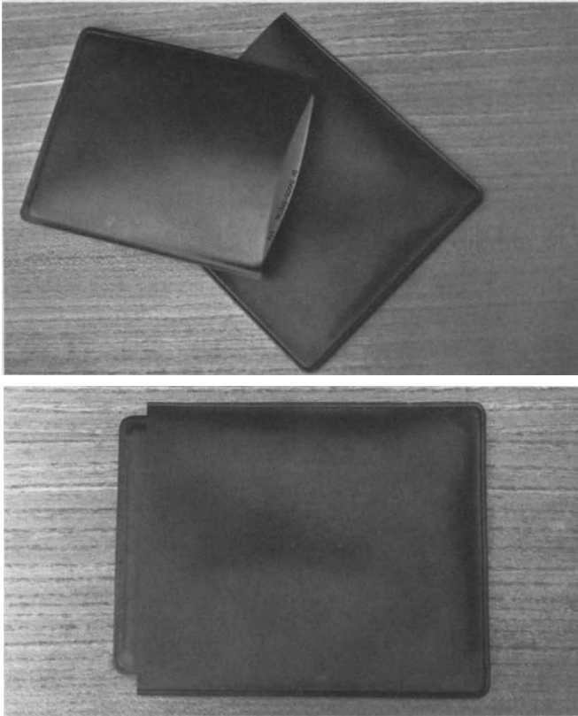
Fig. 4. Telescoping plastic film-wallets made of light-proof plastic and fitted with intensifying screens
