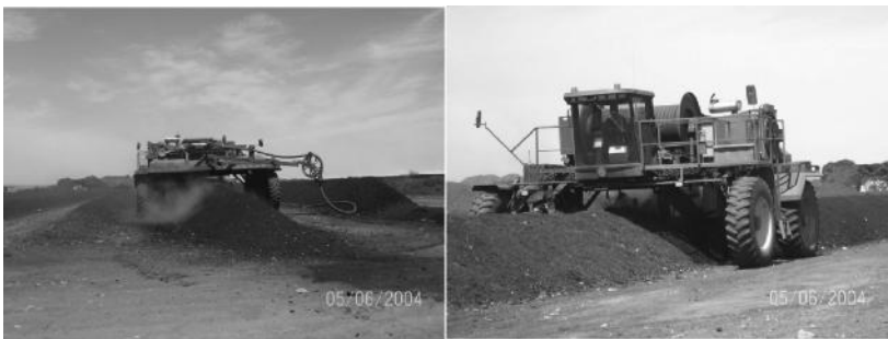
FIGURE 10.1 Spraying water over a windrow during turning. Notice the darker color of the windrow that received the spray.
