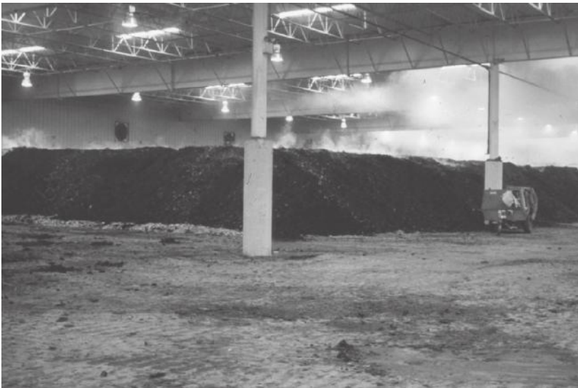
FIGURE 6.8 The inside of the Davenport, Iowa, ASP composting facility. The composting piles are over a trench aeration system.
