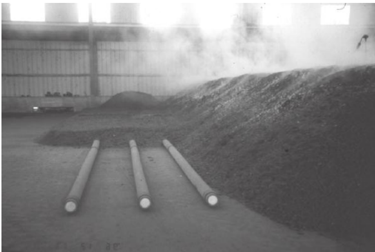
FIGURE 7.16 Aboveground pipes to provide aeration for ASP, showing pipe placement in extended pile.
