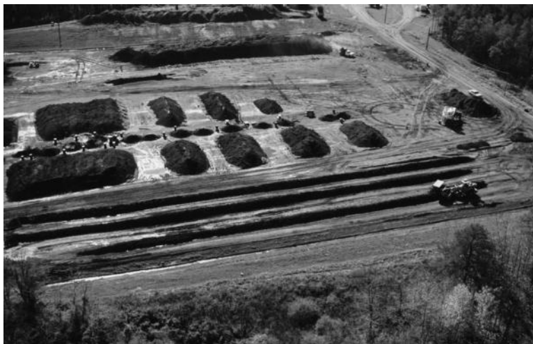
FIGURE 1 Windrow and ASP systems at Beltsville, Maryland. General Motors Terex composter is shown turning a windrow.
