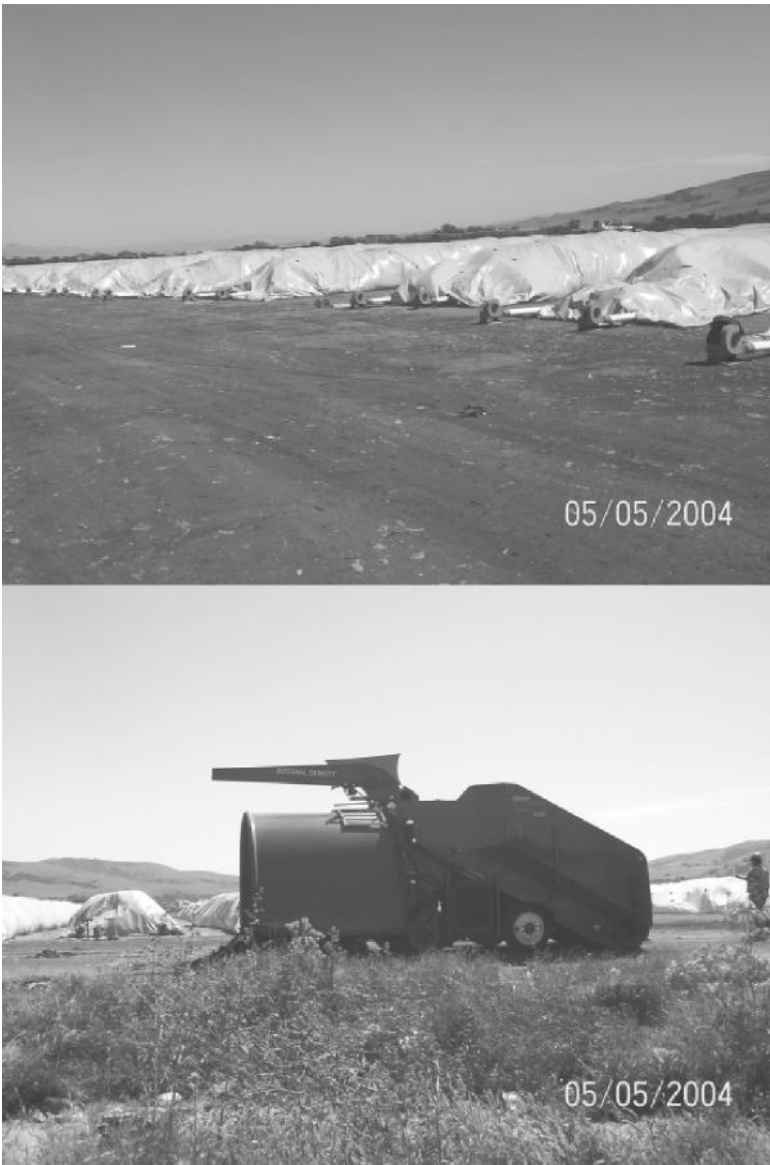
FIGURE 6.17 The Ag-Bag system and loading machine. Aeration provided by blowers.
