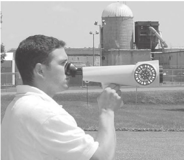
FIGURE 9.12 Using an olfactometer to measure and identify odor sources in the field. (Courtesy of St. Croix Sensory, Inc.)
