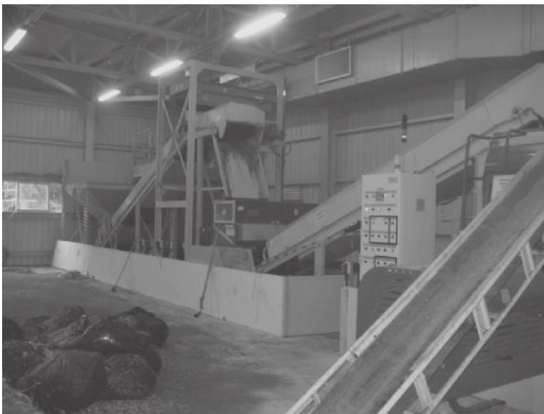
FIGURE 7.10 A Ngau Tam Mei horse manure facility in Hong Kong showing hopper and separation equipment.
