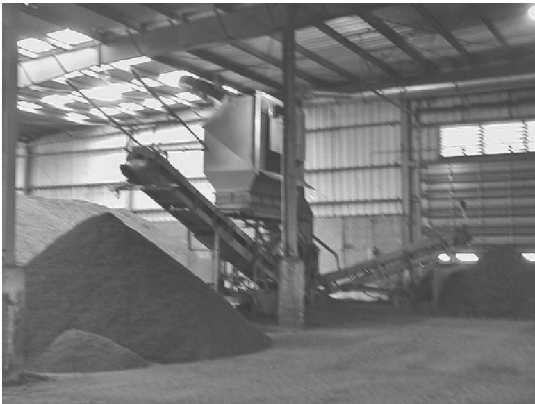
FIGURE 14.2 Dust hood over screen in a composting facility.
