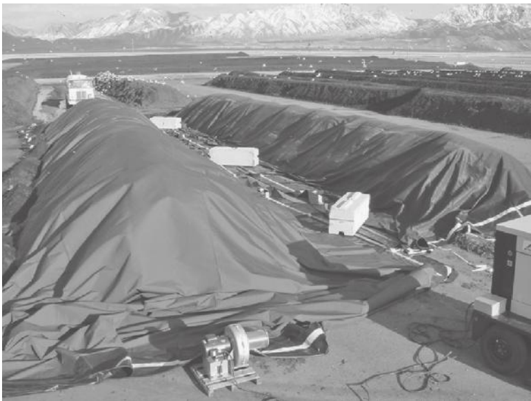
FIGURE 11.13 Managed Organic Recycling (MOR) fabric covers with aerations system in Central Valley, Utah.
