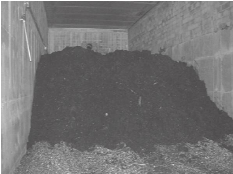
FIGURE 6.11 The material to be composted over an aerated trench system in the bin in Comox, British Columbia.
