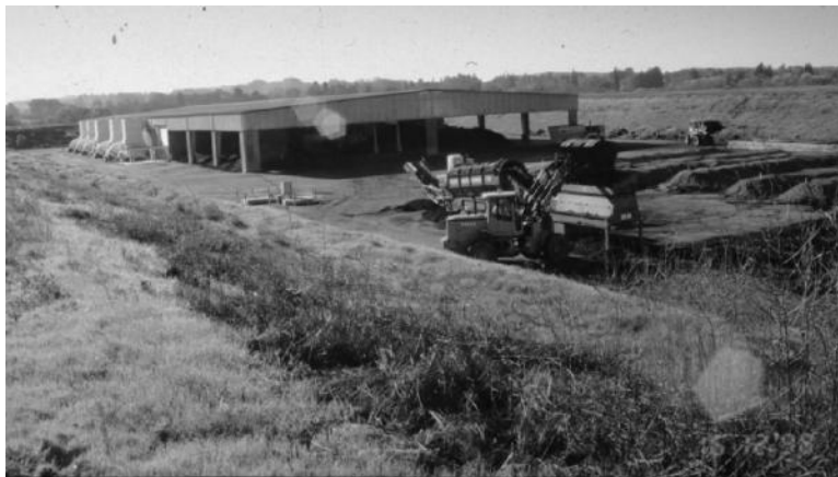
FIGURE 10.3 Use of cover during curing to reduce surface emissions and reduce evaporation in Santa Rosa, California.
