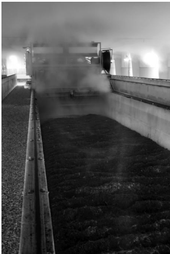
FIGURE 6.21 An IPS agitated bed system in the bay at Greensboro, North Carolina. (Courtesy of Siemens Water Technology Corporation.)
