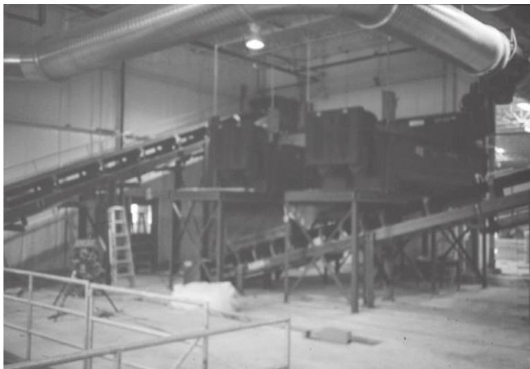
FIGURE 7.6 Pug mills and conveyors at Davenport, Iowa.
