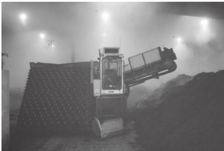
FIGURE 6.20 Windrow turning machine, which lifts the windrow and deposits it along its side. In this case, the unit is used in the LRI enclosed facility.
