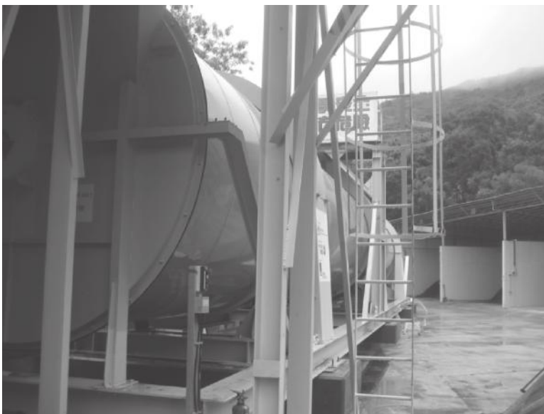
FIGURE 7.11 The drum that follows the processing facility housing the separation equipment. The composting and curing bins are shown in the background.
