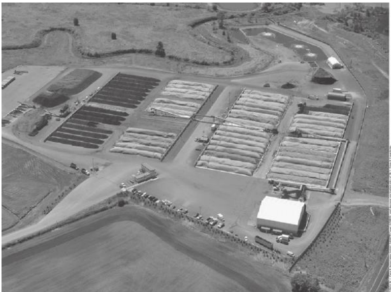
FIGURE 11.15 The Gore fabrics cover system at Cedar Grove composting facility in Washington state. (Courtesy of W.L. Gore & Associates, Inc.)
