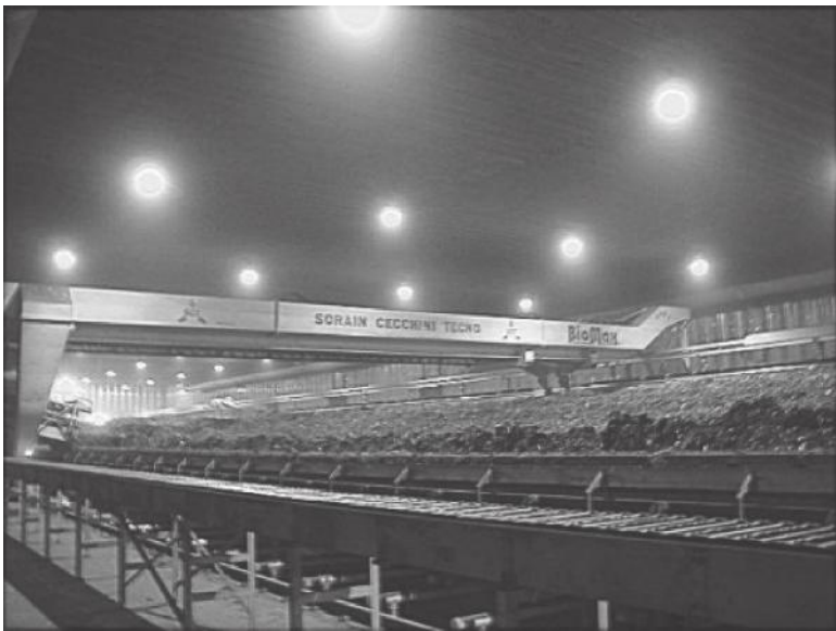
FIGURE 7.9 Edmonton, Canada, MSW and biosolids composting facility, showing the turning machine.
