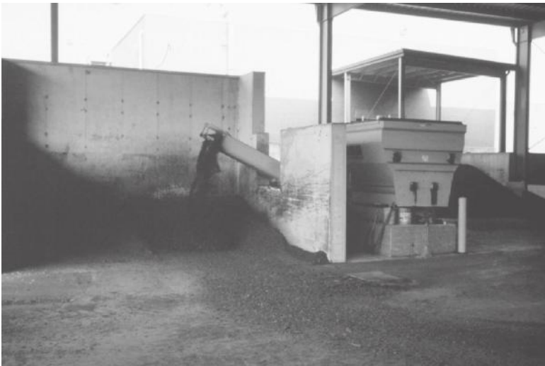
FIGURE 3.5 Stationary mixer depositing biosolids and wood chips into a three-sided concrete bin.
