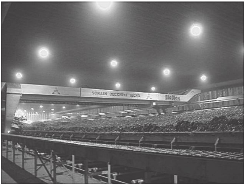
FIGURE 6.25 The Edmonton, Canada, MSW and biosolids composting facility showing the drum and agitated bed system.
