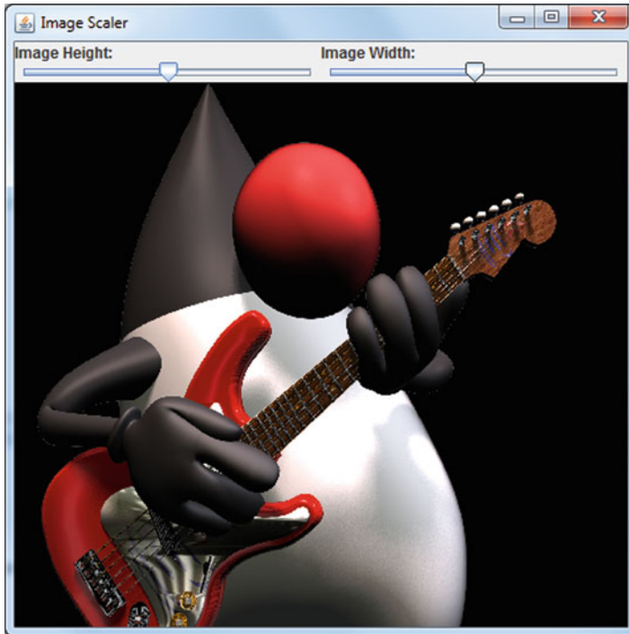
Fig. 18.14 The ImageScaler, showing the scale of an image on one panel controlled by Swing components (in a GridLayout) on a separate panel. Both panels are added to the frame's BorderLayout
