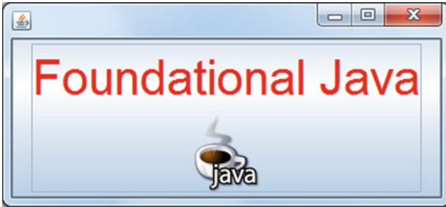
Fig. 17.10 A JButton with an ImageIcon added and its text (in 40 point Helvetica font) positioned at the top and center of the button
