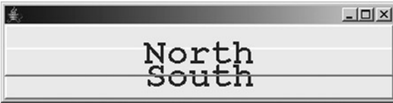
Figure 6-11. BorderLayout vertically resizes the NORTH and SOUTH components as the container height changes
