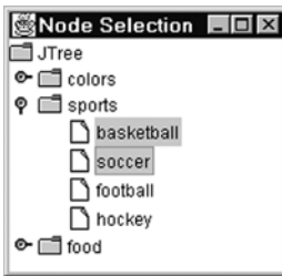
Figure 8-26. How a JTree appears when the basketball and soccer nodes are highlighted
