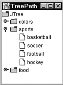
Figure 8-14. To reach the soccer node shown in this tree, you'd need to traverse the JTree , sports , and soccer nodes
