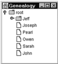
Figure 8-7. By changing the value returned by an object's toString() method, you can control what's displayed for that object when it's part of a tree
