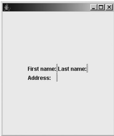
Figure 6-34. GridBagLayout uses preferred sizes if enough space is available but reverts to the minimum size if necessary
