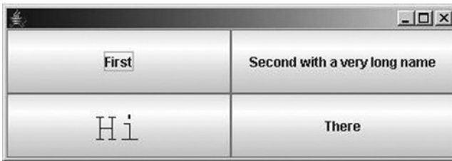
Figure 6-6. GridLayout distributes both horizontal and vertical space evenly to the components regardless of their preferred sizes
