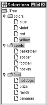
Figure 8-31. Expanding the selected node reveals that its children weren't selected as part of the range selection
