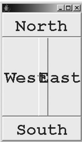
Figure 6-12. BorderLayout horizontally resizes the EAST and WEST components as the container height changes
