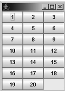
Figure 6-7. You can force GridLayout to use a specific number of columns by specifying a column count but no row count
