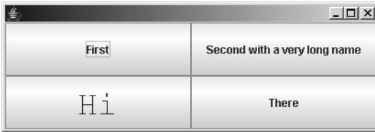
Figure 5-6. GridLayout distributes both horizontal and vertical space evenly to the components regardless of their preferred sizes.
