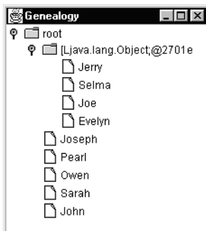
Figure 7-6. Defining a node as an array results in the array elements being represented as children within the tree.
