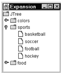
Figure 7-33. You can collapse and expand tree nodes programmatically easily using the methods provided in JTree .
