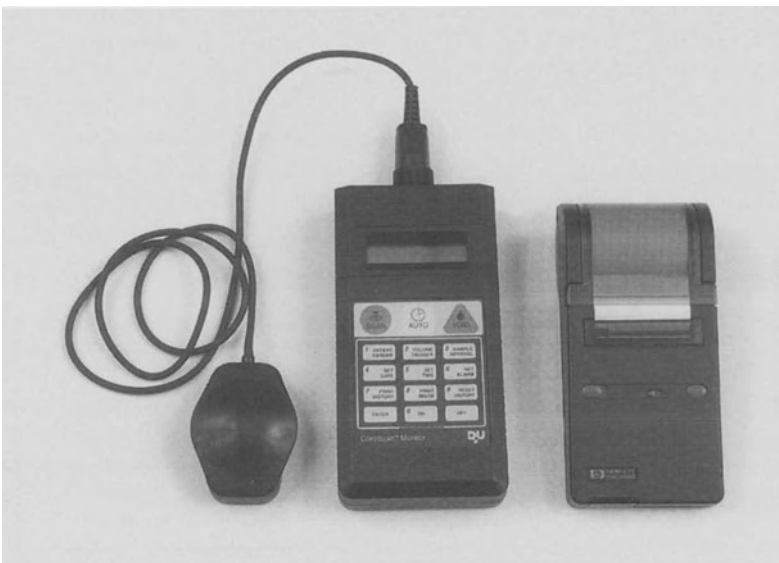
Fig. 3.24 Hand-held or patient-worn ultrasound machine which allows easy recording of bladder volume/post void residual, in clinic, on the ward or in the patient’s home. The photo shows the ultrasound head, the microprocessor with display and a small printer.
