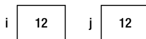
Figure 8-2. Memory overview after declaring and initializing two variables and assigning the value of one to the other
