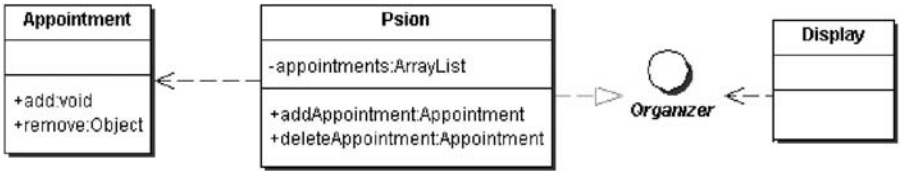
Fig. 3.4 Class diagram produced in Together.
