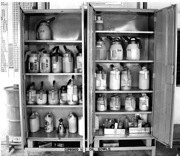
Figure 12.6 Oil dispensing container storage
