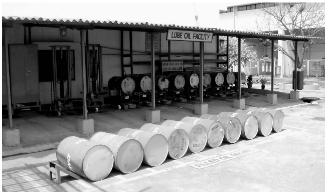
Figure 12.4 Proper storage of oil drums
