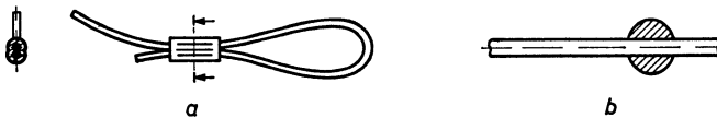
Fig. 1.487. Loop formed on cord with the aid of: a. Crimped metal bush. b. Moulded blob of plastics.
