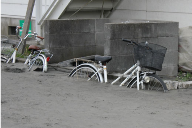
Fig. 10.6 Sand boils and buried cycle
