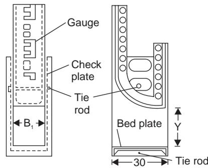
Fig. 3.8 Details of Roof Block
