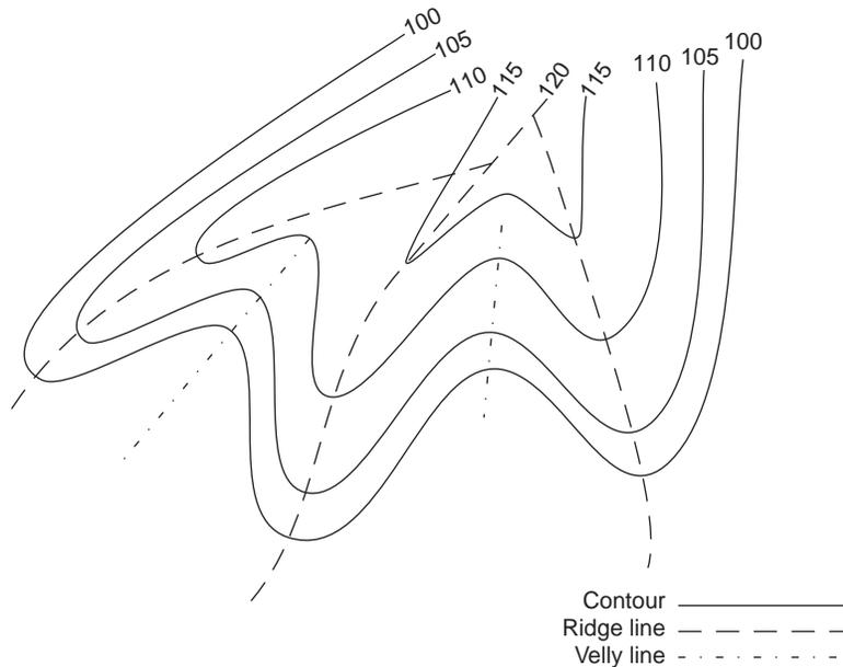
**Fig. 1.6** Water Shed/Sub-Water Shed
