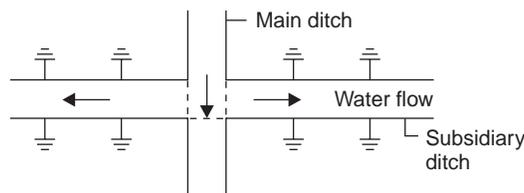
Fig. 1.1 Free Flooding
