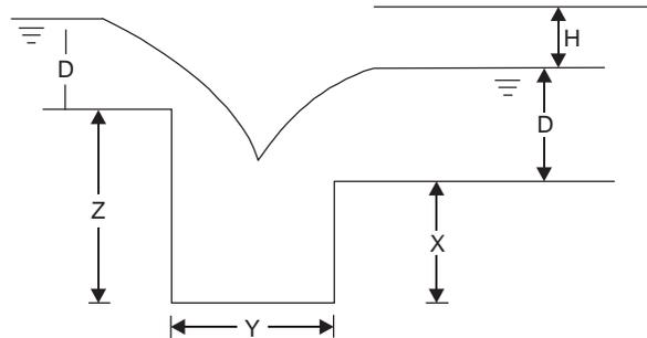
Fig. 7.9 Type Design of a Water Course Fall
