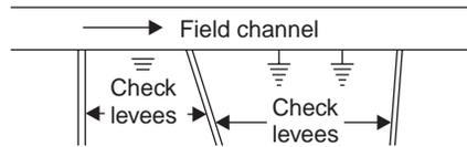
**Fig. 1.3** Check Flooding
