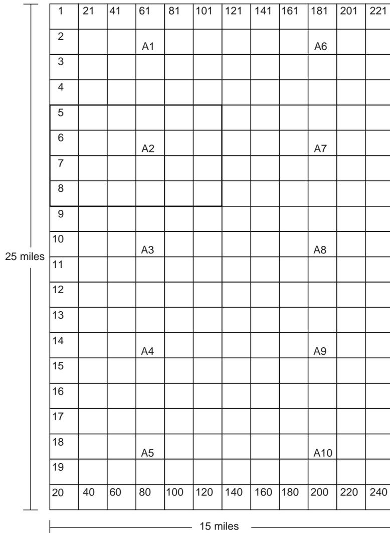
**Fig. 2.3** Arrangement of Survey Sheets
