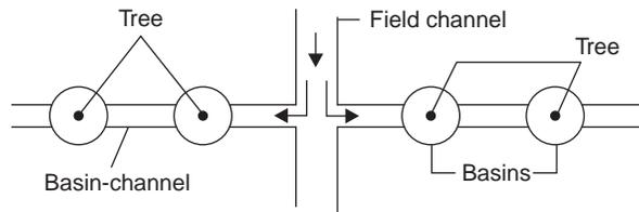
**Fig. 1.4** Basin Flooding
