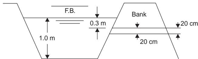
**Fig. 3.7** Submerged Pipe Outlet
