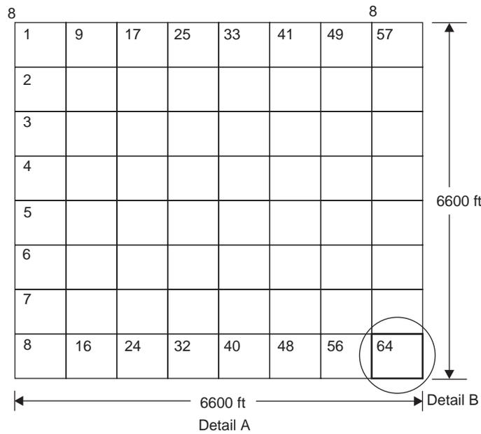
**Fig. 2.4** Rectangulation and Sub-rectangulation
