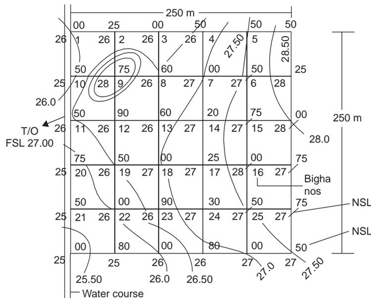
Fig. 7.6 C.C.A. on Weighted Average N.S.L.
