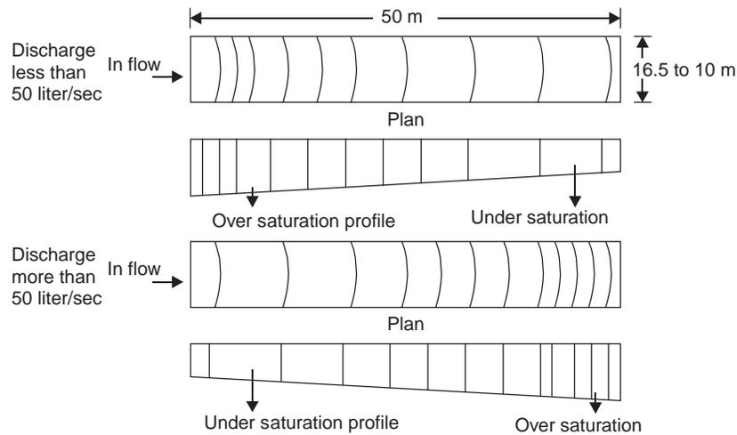
**Fig. 7.1** Over Saturation and Under Saturation Profile
