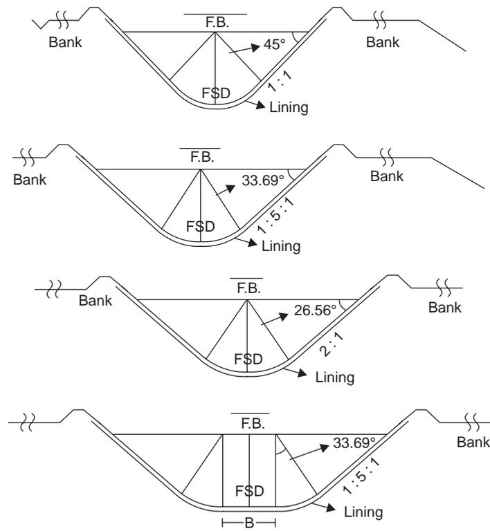
**Fig. 3.3** Semi Circular Canal Section (Mehboob Sections)
