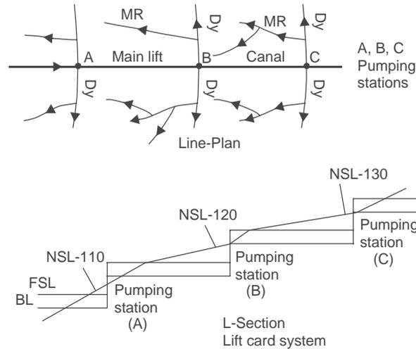
**Fig. 4.2** Lift Canal System
