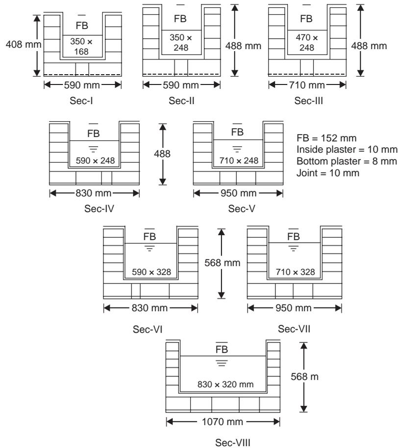
**Fig. 7.8** Brick-Lined-Sections (Brick 23 × 11 × 7.0 cm)
