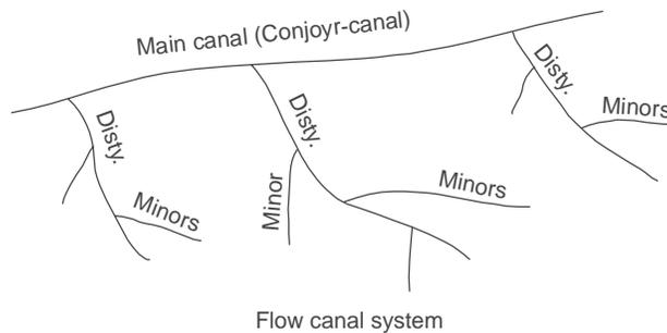
**Fig. 4.1** Flow Canal System
