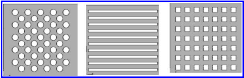
Figure 1. Air inlet grids (from left to right: circle, long and square aperture).
