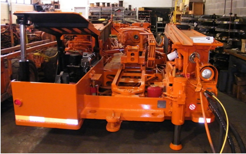
Figure 9.1 The drill unit for in-mine horizontal drilling.
