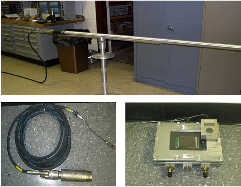
Figure 9.6 The downhole drill monitor.
